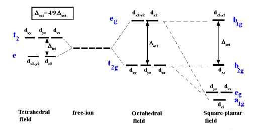
Crystal field d orbital splitting diagrams for common stereochemistries.
